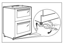
Use small feet on the bottom of appliance to set the appliance top surface level with other surfaces.
