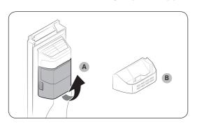
If you do not use the ice maker and need more storage space, remove the icemaker bucket (A). Then, insert the Freezer guide (Optional) (B) into the icemaker bucket's place.
