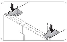
**6.** Insert the hinge covers with the front sides first, and then tighten the screws. Use a Phillips screwdriver for this step.
