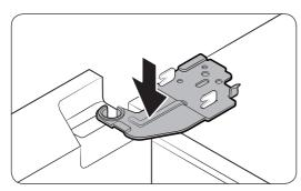
**2.** Put the hinge into its position, and then insert it into the hole on the door.
