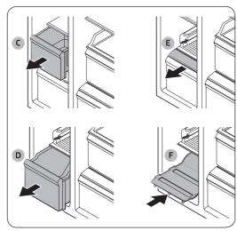
To secure more space, remove the **upper** drawer (C), lower drawer (D), and lower drawer cover (E). Then, insert the provided bottom shelf (F).
