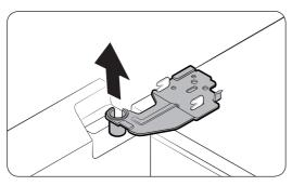
**6.** Open the door by 90 degrees. While holding the door, remove the hinge.
