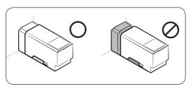
**3.** Reinsert the water tank and fit into the dispenser mechanism. Make sure the front side (with the front lid) of the tank faces to the front.
