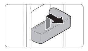
To remove a door bin, hold the front sides of the bin and gently lift up to remove.
