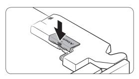
**4.** Insert the upper area of the adapter cover first, and then close to lock as shown.
