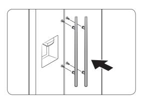
**1.** Attach the handle supports on the brackets.
