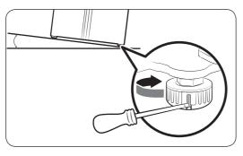
To adjust the height of the fridge side: Insert a flat-head screwdriver into the leveller of the fridge-side front leg. Turn the leveller clockwise to raise, or turn it counter clockwise to lower.
