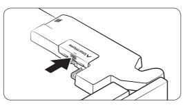
**1.** Press to unlock the arrow area of the adapter cover.
