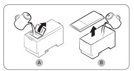
2. Open the front lid (A) of the cover or the entire cover (B) and fill the tank with a max of 5 litres water.
