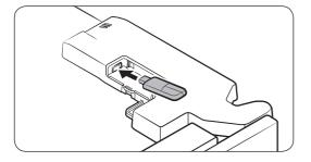
**3.** Insert the Smart Home Adapter into the adapter port in the correct direction.
