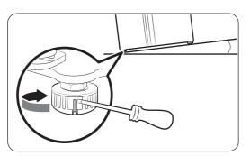
To adjust the height of the freezer side: Insert a flat-head screwdriver into the leveller of the freezer-side front leg. Turn the leveller clockwise to raise, or turn it counter clockwise to lower.
