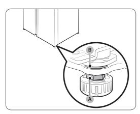
Open the door to adjust, and locate the two nuts (A) and (B) on the front bottom of the door.
