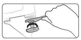
**3.** When levelling is complete, tighten the nuts using the spanner.
