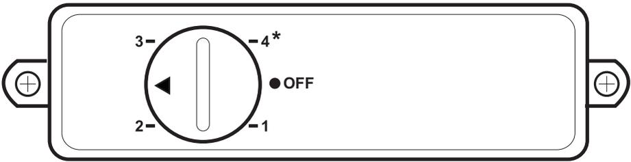
Temperature is controlled by the thermostat which is located on the rear wall of the cabinet (see the diagram on page 5). Thermostat knob is located on the thermostat housing. "Number 4" is the coldest setting. The normal storage temperature of your appliance should be  $-18\text{ }^{\circ}\text{C}$  ( $0\text{ }^{\circ}\text{F}$ ). Lower temperatures may be obtained by adjusting the thermostat knob towards 'number 4' position.
