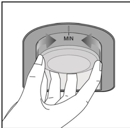
Operating temperatures are controlled by the thermostat knob (see diagram) located on the ceiling of fridge compartment. Settings may be made from **MIN**, 1 ... **MAX**, **MAX** being the coldest position.
