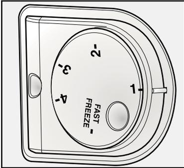
Operating temperatures are controlled by the thermostat knob (see diagram) located on the inner side wall of the freezer compartment. Settings may be made from 1, 2 ... fast freeze, fast freeze being the coldest position.
