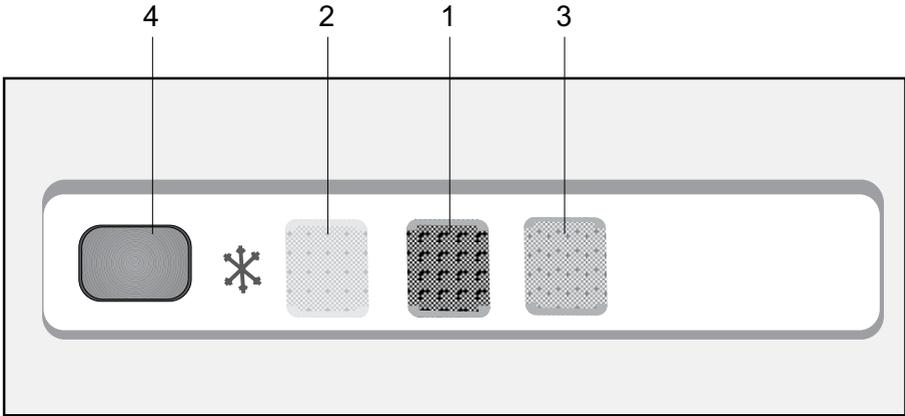
Temperature is controlled by the thermostat which is located on the rear wall of the cabinet. Thermostat knob is located on the indicator light set. "Number 4" is the coldest setting. The normal storage temperature of your appliance should be  $-18\text{ }^{\circ}\text{C}$  ( $0\text{ }^{\circ}\text{F}$ ). Lower temperatures may be obtained by adjusting the thermostat knob towards 'number 4' position.
