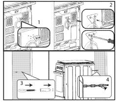
Stability chain to be as short as practicable to avoid oven tilting forward and diagonal to avoid oven side tilting.
