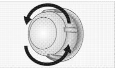
3. If your oven lamp is of type (A) shown in the figure below, remove it by rotating as shown and replace it. If it is of type (B), pull and remove it as shown in the figure and replace it.
