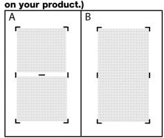
When the two separate cooking zones (shown in the figure A) are combined as a wide surface cooking zone shown in the figure B, the separating light should go off. When the wide surface cooking zone is returned back into two separate cooking zones, the separating light should be illuminated.
