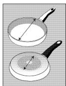
Some saucepans have a smaller ferromagnetic area than the real diameter of the saucepans, Only this area will be heated up by the induction zone. therefore the cooking performance may be reduced. These pan types cannot be detected by bigger induction zones. The diameter of pan's ferromagnetic area should match the size of the cooking zone. If the pan is not detected by the cooking zone, try it on the next smaller cooking zone.
