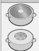
Some vessels have a base which includes nonferromagnetic materials such as aluminum. These types of vessels cannot be detected by the induction zone.
