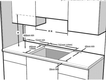
Minimum height to extractor as recommend in extractor instruction manual \*\* Minimum distance between cabinetry must be equal to width of hob
