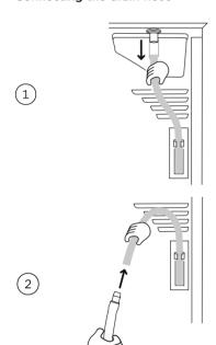
Remove the black hose from the connection at the back of the dryer.
