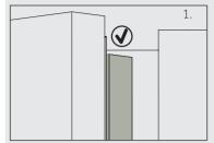
When you close the door, the vertical door strip on the left door should be bent inside (1).
