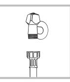
1. Connect the supply pipe by screwing it to a cold water tap using a 3/4 threaded connection (see figure). Before performing the connection, allow the water to run freely until it is perfectly clear.
