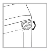
2. If the floor is not perfectly level, compensate for any unevenness by tightening or loosening the adjustable front feet (see figure); the angle of inclination, measured according to the worktop, must not exceed 2°. Levelling your appliance correctly will provide it with stability and avoid any vibrations, noise and shifting during operation. If it is placed on a fitted or loose carpet, adjust the feet in such a way as to allow enough room for ventilation beneath the washing machine.
