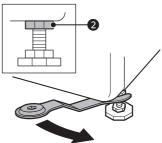
Check if all lock nuts at the bottom of the appliance are secured properly.
