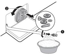
After cleaning the drain pump filter, carefully reinsert the filter and screw the drain cap back in clockwise carefully to avoid cross threading
