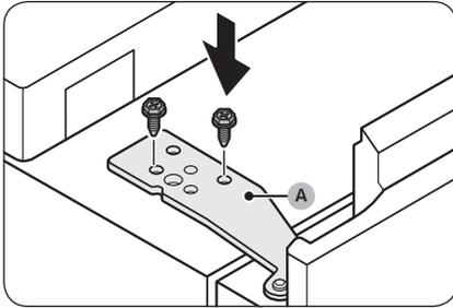
29. Fasten the **top hinge (A)** with the screws using a socket wrench (10 mm).
