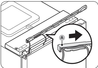
38. Place the wire from the fridge door into the space underneath the **wire cover (A)**.
