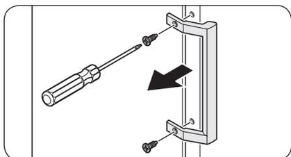
2. Use a Phillips screwdriver to remove the screws and detach the handle.
