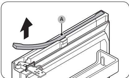
22. On the top of the fridge door, remove the **wire cover (A)**.
