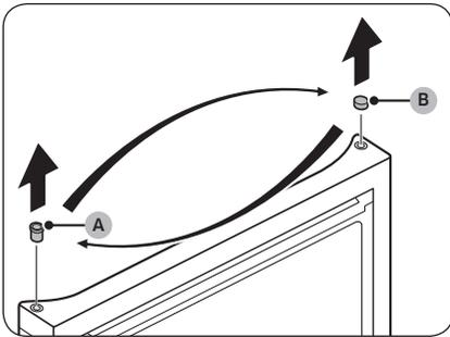
14. On the top of the freezer door, switch the position of the **grommet (A)** and the **grommet cover (B)**.
