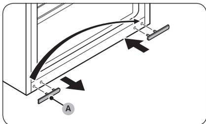
12. Remove the **bottom hinge screw cover (A)** and put it on the opposite side.
