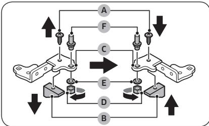
16. Disassemble the bottom hinge and reverse all the parts.
