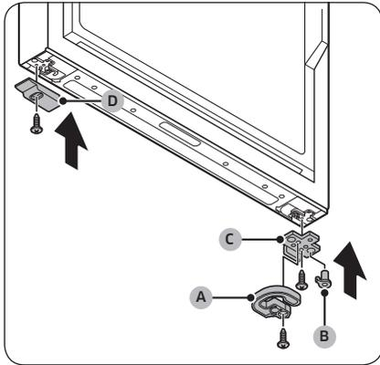
21. Switch the sides of all the removed parts.
