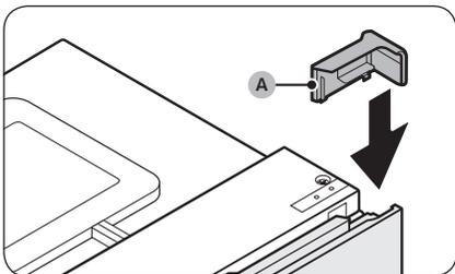
37. Put the provided **top-right door cover (A)** on the opposite side of the door hinge.
