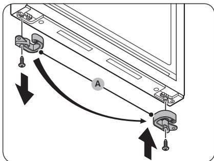
13. On the bottom of the freezer door, remove the **door stopper (A)** and put it on the opposite side of the door.
