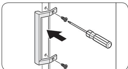
4. Place the handle on the opposite side of the door and use a Phillips screwdriver to attach the handle with the screws.
