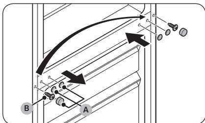
10. Remove the **middle hinge screw covers (A)**, and then use a Phillips screwdriver to remove the **screw (B)**.
