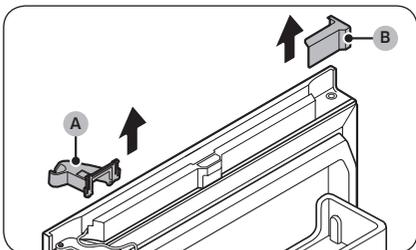
23. Remove the **top-right hinge cover (A)** and the **top-left door cover (B)**.
