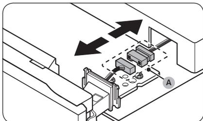
4. Disconnect the **wire connector (A)**.
