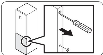
3. On the opposite side of the door, use a flat-head screwdriver to remove the screw covers.
