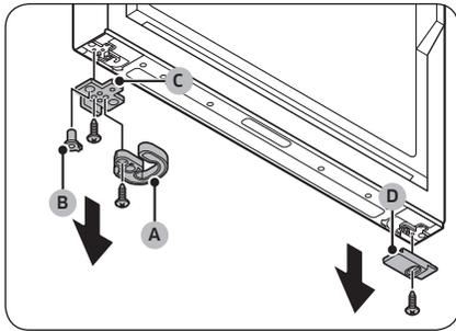
20. On the bottom of the fridge door, remove all the part on the left and right side.
