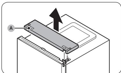
2. Gently lift the **top cover (A)** and place it on top of the refrigerator.
