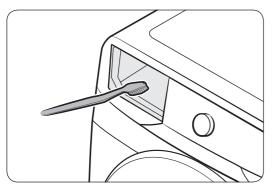
**3.** Clean the drawer recess using a bottle brush to remove detergent residues and limescale on the drawer recess.
