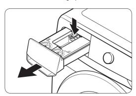
While holding down the release lever on the inner of the drawer, pull the detergent drawer to remove.
