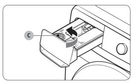
**4.** Turn the **auto softener compartment cover (C)** anticlockwise to open.
