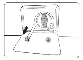
**3.** Put an empty, spacious container around the cover, and stretch the emergency drain tube to the container while holding the **tube cap (A)**.
