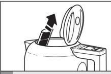
To access filter: Open the lid; the filter is located behind spout inside Electric Kettle. Grasp the top of the filter to remove.
