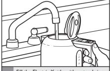
Fill the Electric Kettle with water, bring to a boil and drain out the water. Repeat this step twice. The Electric Kettle is now ready to use.
