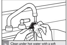
brush or cloth to remove deposits, and replace filter by sliding the filter into the slot behind the spout.
