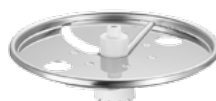
Externally adjustable slicing disc with integrated wiper Slices are perfectly cut; change the thickness instantly by using the external lever. The food wiper, that is fixed under the disc, pushes food towards the opening while slicing.
