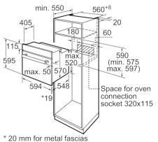
measurements in mm
