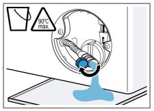
9. Firmly press on the sealing cap.
