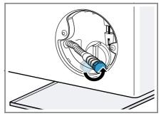
10.Insert the drain hose into the holder.
