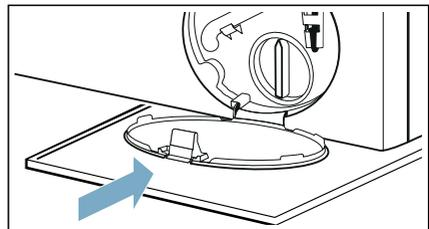
**Note:** To prevent unused detergent from flowing straight into the drain during the next wash: Pour 1 litre of water into dispenser II and start the **Drain** programme.
