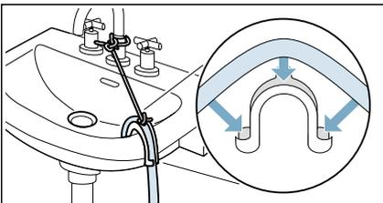
■ **Drainage into a plastic pipe with rubber bushing or into a drainage pit**
