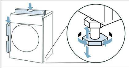
3. Tighten the lock nut against the housing. In doing so, hold the foot tight and do not adjust its height. The lock nuts on all four appliance feet must be screwed tightly against the housing.
