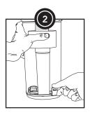
Push the release button, open the dust canister and clean all parts of the dust canister.
