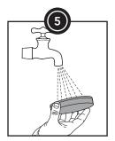
Use cold running water (no detergents) to wash both parts of the filter.
