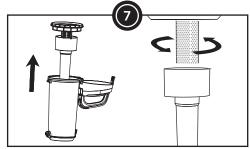
Lift out the assembly from transparent dust canister and then untwist filter from the central tube to remove for cleaning dirt and debris as needed. Follow steps in reverse to reassemble.
