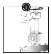
Close the base of the dust canister, align the canister base back onto the machine and push until it clicks back into place.
