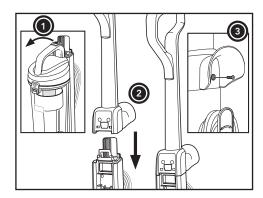
Remove the dust canister before installing handle. Push the handle onto the vacuum body, and use a Phillips screwdriver to secure it with the screw provided.
