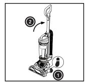
Step on the brush cover and pull back on handle, to engage for operation.
