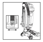
Place the short hose end onto the connector (left hand side if looking at the back of the vacuum), and rotate clockwise to lock.
