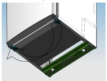
6) Set the door right position ,fix the mid-hinge .
