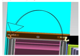
8) Set the top door right position , fix the top-hinge and the cover.
