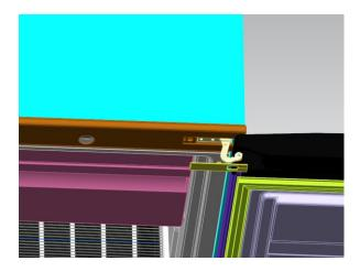
2) Remove the screws fixed the top-hinge with cross-slot screwdriver.
