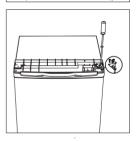
4. Unscrew bottom hinge. Then remove the adjustable feet from both side.
