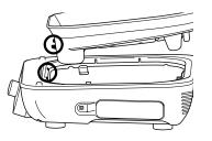
2 Place flat plate on the grill so plate sits level. Line up the lip on the flat plate with the lip on the grill plate (if incorrectly installed it will tilt forward). Close the lid.
