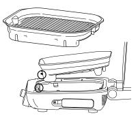
2 Place the crisper basket on the plate and position the basket to sit along the rear of the grill plate so the basket feet sit in the grill plate spaces. Add ingredients, then close the lid.
