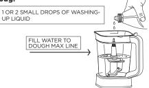
With the dough or stacked blade assembly installed, fill with warm water up to DOUGH MAX line and add 1 or 2 small drops washing-up liquid. Secure jug lid and ensure the pour spout is securely closed.
