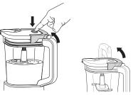
8 Remove the lid and Dough Blade Assembly before removing contents. To remove the lid, press the **RELEASE** button and lift the handle. To remove the blade assembly, carefully grasp it by the top of the shaft and pull straight up. The jug can then be emptied.
