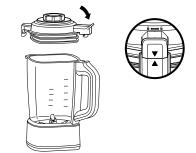
**5** Secure the centre cap by placing it down into the lid and twisting clockwise until it clicks into place.
