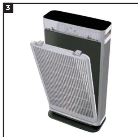
3. With the filter installed, replace the filter cover. Insert the tabs on the bottom of the cover into the slots on the unit. Press the top of the cover, then the sides, until it clicks into place. **DO NOT** run the air purifier unless the filter is removed from its packaging and installed correctly.
