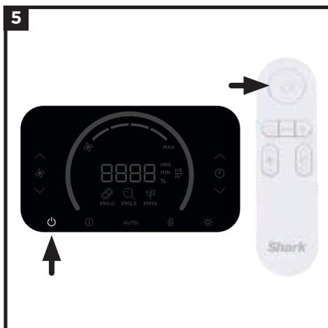
5. Plug the unit into an electrical outlet and press the power button on the top control panel or on the remote.
