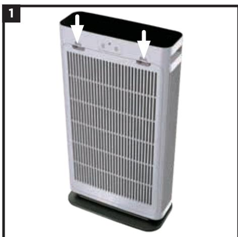
1. Before plugging in the unit for the first time, you must remove the filter and take it out of its packaging. First, remove the filter cover from the back of the unit. Press the tabs near the top and pull the cover toward you.
