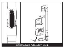
To put the vacuum in storage mode, press the **Unlock** latch while folding the handheld vacuum forward until the wand clicks and locks. Plug the charger into the charging port on the handheld vacuum.
