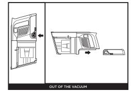
To remove the battery, squeeze the **Battery** Release Button and slide backwards. Plug the charger into the charging port on the battery.
