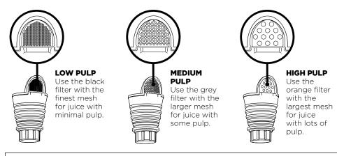
**NOTE:** For best results, we recommend using the **Grey (Medium Pulp)** or **Orange (High Pulp) filter** when processing soft fibrous fruits like berries, seeded melons and pineapple.
