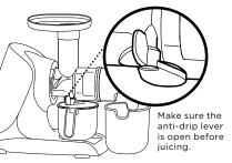
6 Place the pulp container under the pulp spout, then place the juice jug under the anti-drip lever on the feed chute chamber.
