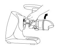
**9** To disassemble, press and hold the RELEASE button while turning the feed chute chamber clockwise and remove from motor base.
