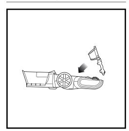
**4** To reassemble, replace base by lining it up along the front of the nozzle. Push down to snap into place. Lock the 3 locks.
