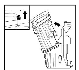
Pull up on **Dust Cup Release Latch** on the handle and lift dust cup off pod.
