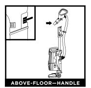
Press the **Handle** button to detach the handle from the wand.
