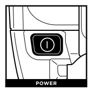
Press power button to turn the vacuum on or off. Please note the brush-roll will not spin unless the wand is reclined.
