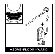
Press the Wand Release button to detach the wand from the pod.
