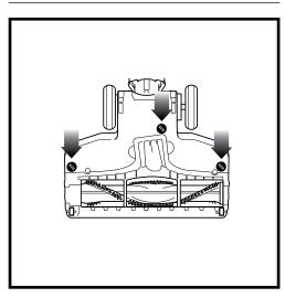
1 Use a coin to unlock the 3 locks on the bottom of the floor nozzle.
