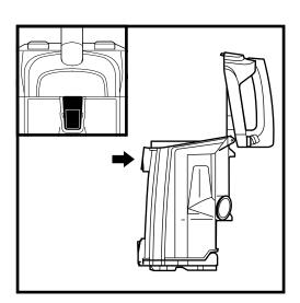
Press Top Empty Release Latch to access dust screen and remove built-up debris as necessary.
