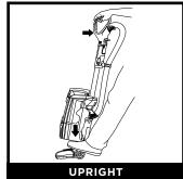
To engage brush-roll, turn on power, then step on the floor nozzle and tilt the handle back.
