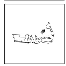
2 A portion of the base is removable to allow for better access to the brush-roll and exposure to the airway. Shine a torch from the bottom to check for possible blockage in the airway.
