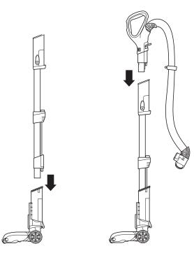
1 Place motorised floor nozzle on floor and insert wand, pressing it in until it clicks securely into place. 2 Insert handle into wand, pressing it in until it clicks securely into place.
