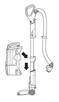
3 Place pod onto wand and slide down to connect.
