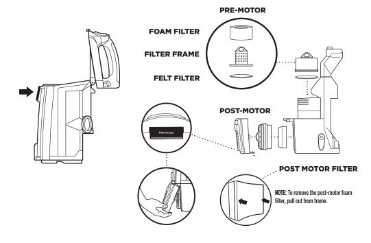
**3** Press top dust-cup empty latch to access dust screen and remove built-up debris as required.
