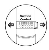
**3** The Suction Control slide. located at the base of the top handle. offers variable suction based on your needs. Slide toward MIN to minimise suction, and slide toward MAX to maximise suction.
