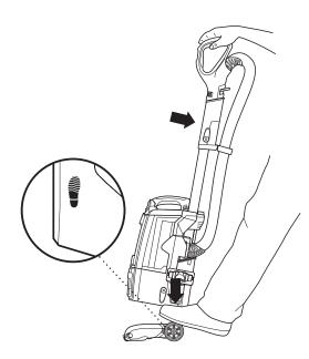
1 Plug power cord into socket. Place foot on floor nozzle and tilt handle back.
