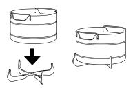
1 To remove diffuser for cleaning, pull 2 diffuser fins off the groove on the basket, then pull diffuser down firmly.
