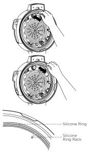
To remove the silicone ring, gently pull it outward, section by section, from the silicone ring rack. The ring can be installed with either side facing up. To reinstall, press it down into the rack section by section, (see image above).
