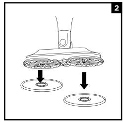
2 To attach the Dirt Grip<sup>™</sup> pads, place **BOTH** the pads flat on the floor with the plastic rings facing up. Align the indentation on the rotating discs on the bottom of the nozzle with the plastic rings on the pads, then gently lower the nozzle onto the pads, pressing until the pads are secured.
