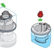
Remove the cap and fill tank (no other part) to the top with cold tap water. Replace the cap, tank and loop amplifier. Use the handle for easier handling.
