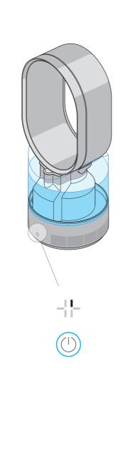
Switch 'ON'. The water treatment procedure automatically starts. Water passes over a UV-C emitter to ensure that it is 99.9% bacteria-free before misting commences. This takes approximately 3 minutes. (During this time humidity targets can be set and fan mode can be switched ON'.)
