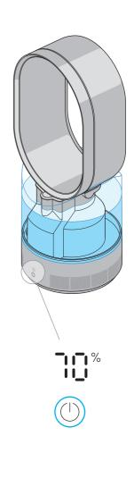
After 3 minutes the appliance will start to humidify. The display will show the target humidity setting.
