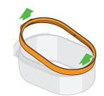
Unclip the loop amplifier surround: pull from the lower edge by hand, gently but firmly.
