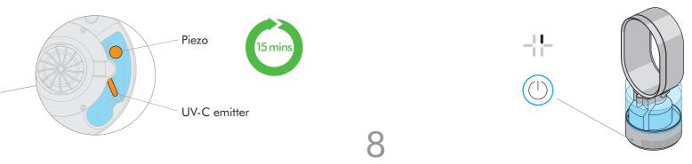
dishwasher. Fill the trough with the recommended acid citric solution until the UV-C emitter and piezo are submerged. Leave for 15 minutes. Drain, rinse and wipe over all surfaces. Repeat if necessary.
