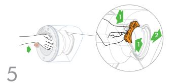
To remove the seal, pinch the securing tabs together and pull out. Clean thoroughly by immersing in the recommended citric acid solution for 15 minutes. Rinse and wipe over all surfaces. Repeat if necessary. To refit, push back in so the tabs click and the fit is secure. **3** To attach the loop amplifier surround, lie flat and align the surround to the main amplifier. Push firmly until it clicks into place as shown.
