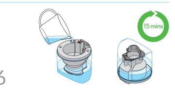
Pour in the recommended citric acid solution. Replace the cap and shake tank for 30 seconds. Then leave to stand. After 15 minutes, empty the tank. Rinse and wipe over all surfaces. Repeat if necessary.
