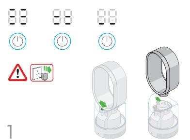
Unplug the appliance and push the button to unlock. Lift the loop amplifier away from tank, then tank away from base.
