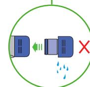
Check that the filter unit is completely dry.
