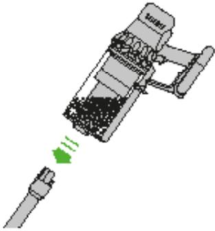
Press the red wand release button and pull the wand away from the bin.
