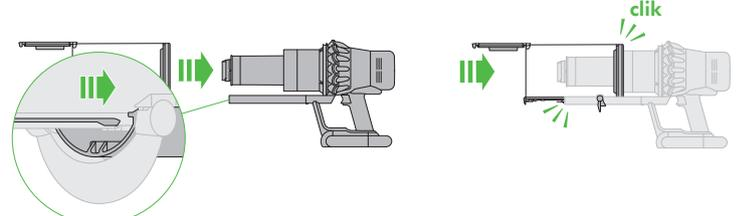
To refit the bin, insert the spine on to the bin runner.
