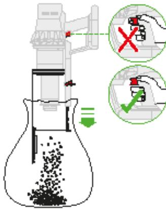
To release the dirt: Hold the machine over the bin in a downwards position.
