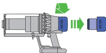
Remove the filter unit by twisting it anti-clockwise. Gently pull it away from the machine.
