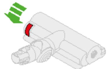
The cleaner head housing is not washable and should only be wiped over with a damp lint-free cloth.
