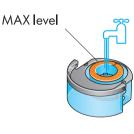
Place the evaporator in the water tank. Fill the water tank to the Max level with cold tap water.
