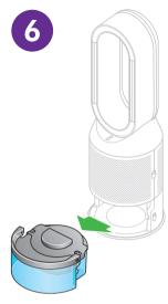
When the LCD screen shows the Deep clean cycle is complete, push down the water tank release buttons on the sides of your machine.
