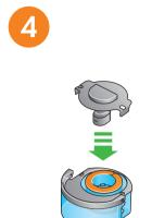
Replace the cap and secure the cap clips in place.
