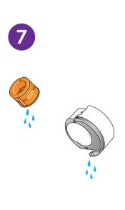
Unclip the cap, take the evaporator out of the water tank and rinse under a cold tap.
