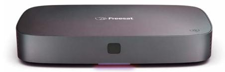
The purple light means the Box is transitioning between standby and on.
