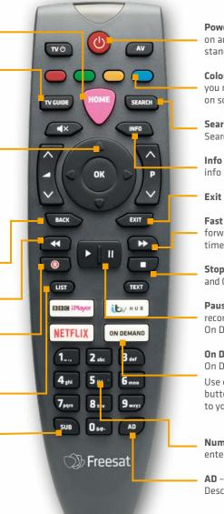
**Power** – turns the Box on and puts it into standby mode
