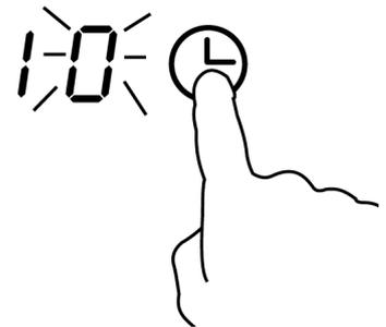
3. While the units digit is flashing, use the slider control to select the units digit of the minute minder duration time.
