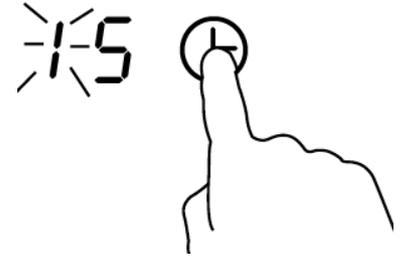
5. While the tens digit is flashing, use the touch control slider key to set the tens digit of the cooking duration time, e.g. 9 in this example to make 95 minutes in total.
