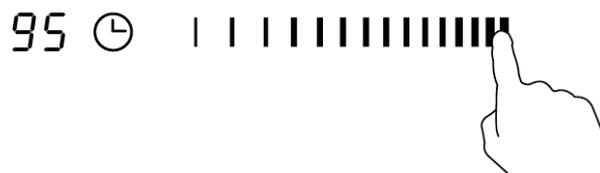
6. After a few seconds, the tens digit of the minute minder duration time is accepted and the minute minder duration time starts to count down in the display.
