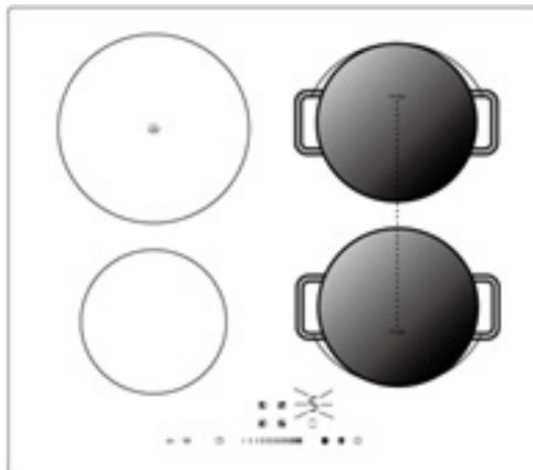
**Note:** Ensure that the magnetic bases of the pans have a diameter of at least 140mm.
