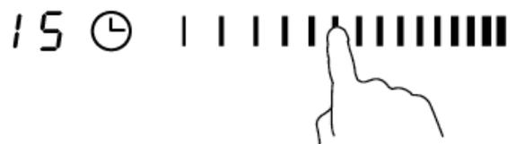
4. Touch the timer control key again. The units digit is accepted and the tens digit starts flashing.
