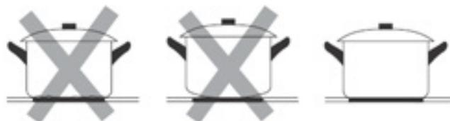
Make sure that the base of your pan is smooth, sits flat against the glass. Use a pan which is at least as large as the circle printed on the glass. Using a pan which is slightly wider than the glass circle printed on the glass will maximise energy-efficiency Always centre your pan on the cooking zone.
