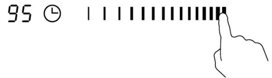
6. After a few seconds the tens digit is accepted and the cooking duration time starts to count down in the display. A red dot flashes next to the relevant cooking zone power level indicator, to show that the zone is currently being controlled by the timer.
