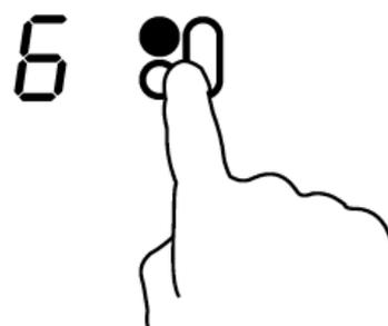
2. Touch the heating zone selection control of the relevant zone again to ensure that it is selected, and make sure that the power level indicator next to the zone is flashing. While the power level indicator is flashing, touch the timer control key. The timer display shows the default time of 10 minutes, with the units digit flashing.
