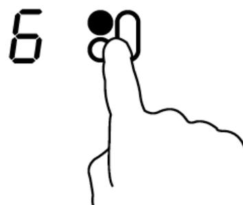
While the power level indicator is flashing, use the slider control to turn the power level down to 0. The zone switches off.
