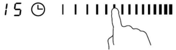
4. Touch the timer control key again. The units digit is accepted and the tens digit will start flashing.
