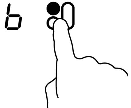
2. While the power level indicator is flashing, touch the power boost control key to cancel the power boost function. The zone will revert to the on-going power level.
