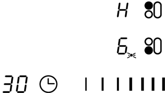
If you want to see how long a zone has left to run, touch the heating zone selection control key for the relevant zone and the time remaining will be displayed briefly on the timer display.
