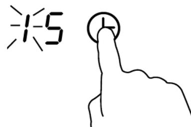
5. While the tens digit is flashing, use the slider control to select the tens digit of the minute minder duration time.
