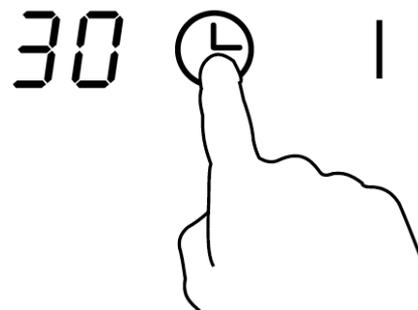
3. While the timer display is flashing, use the touch control slider to adjust the cooking duration time down to 00.
