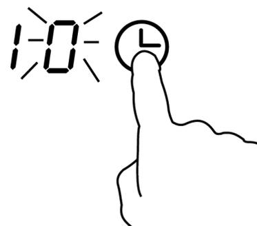
3. While the units digit is flashing, use the touch control slider to set the units digit of the cooking duration time, e.g. 5 in this example.
