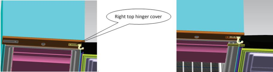
2) Remove the screws fixed the top-hinge with cross-slot screwdriver.
