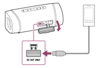
When you connect the speaker to an AC outlet, the connected USB device starts to be charged automatically. If the speaker is being powered by the built-in battery only, proceed to step ②.
