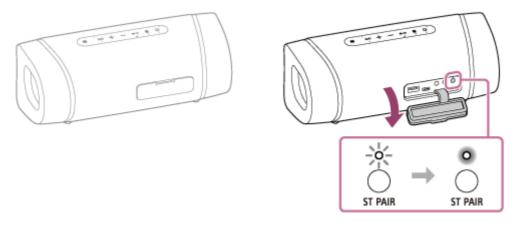
When a connection with the Stereo Pair function is established, the ST PAIR (Stereo Pair) indicators on both speakers stay lit and the (BLUETOOTH) indicator on either of the speakers turns off.
