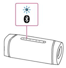
After you pair the speaker with a BLUETOOTH device for the first time since purchase or initialize the speaker (the speaker has no pairing information), the speaker automatically enters pairing mode when it is turned on. Proceed to step 4.
