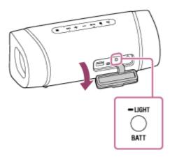
By pressing and holding the button for about 3 seconds again, the lighting function turns on/off again.
