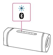
After you pair the speaker with a BLUETOOTH device for the first time since purchase or initialize the speaker (the speaker has no pairing information), the speaker automatically enters pairing mode when it is turned on. Proceed to step  $\S$  .
