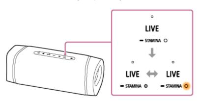
If you press and hold the LIVE/ — STAMINA button for about 3 seconds once again, the STAMINA indicator will turn off and the sound effect will be switched back to EXTRA BASS mode.
