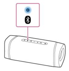
The speaker has been connected to the BLUETOOTH device.
