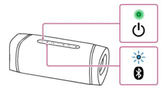
When the speaker has no pairing information, for example when you use the BLUETOOTH function for the first time after purchase, the \( \begin{align\*} \) (BLUETOOTH) indicator keeps double flashing in blue.
