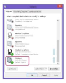
If you cannot click [Connect] for [SRS-XB33 Stereo], select [Disable] for the [Default Device] that currently has a checkmark (green).
