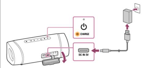
The CHARGE indicator lights up in orange while charging is in progress.
