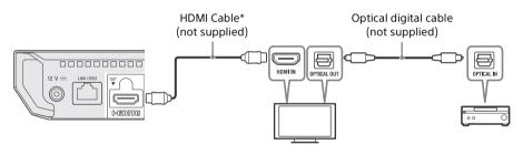
\* A Premium High Speed HDMI Cable or High Speed HDMI Cable that supports 18 Gbps bandwidth.
