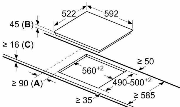
**A:** Minimum distance from the hob cut-out to the wall.**B:** Recessed depth**C:** With fitted oven underneath min. 20, possibly more; see space requirements for the oven.
