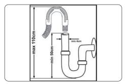
Connect the water drain hose directly to water drain hole or to the sink outlet spigot. This connection should be minimum 50 cm and maximum 110 cm from floor that dishwasher is placed.
