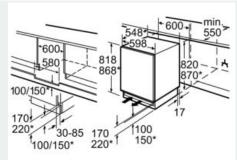
\* variable base/substructure height
