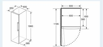
measurements in mm
