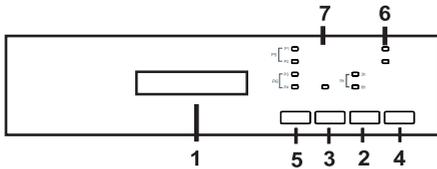
By pressing On/Off button (4), energise the machine. On/Off lamp lights as long as the machine is on. Select the suitable programme by pressing Program button (5).
